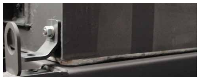
Illustration 2: Boiler attachment on fireplace body
