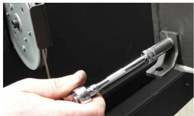
Illustration 1: Mounting bracket removal
